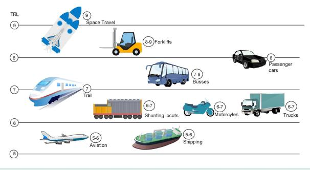
Figure 8: Technology maturity levels (TRL) of mobile hydrogen applications
