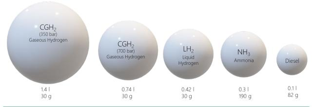
Figure 1: Volumetric and gravimetric energy density of fuels (drop sizes with fixed energy content of 1 kWh)
