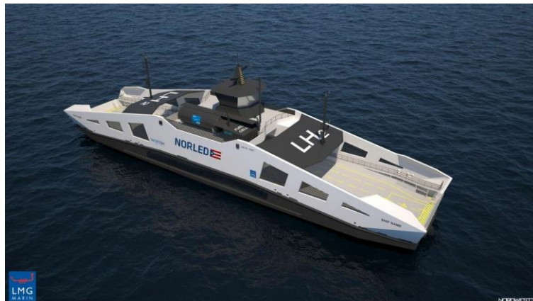
Figure 6: Norwegian Ferry utilizing LH 2 for propulsion [7]
